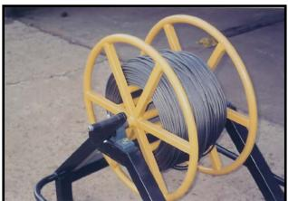
The 1 ton cable pulling winch has been designed to accommodate easy maneuverability on site, in buildings and manholes. The base frame is generally designed to fit customer requirements. This will included fitting on LDV's, different manhole sizes, indoor cable pulling applications, vertical up and down cable pulling operations as well as general horizontal pulling operations.
